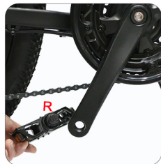
The pedal "R" is installed on one side of the chainring, and "L" is opposite to the chainring
