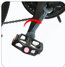
Tighten the right pedal "R" clockwise
