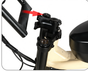
Install the handlebar to adjust the direction
