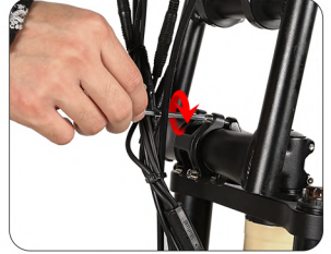
Tighten 4 screws to fix the handlebar
