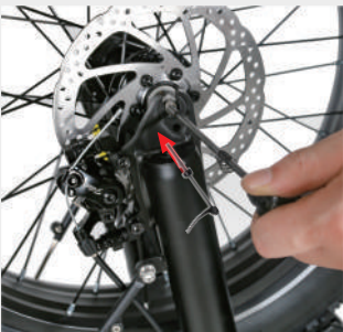
Place the quick release clamp into the front wheel clamp slot
