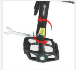
Tighten the left pedal "L" counter clockwise
