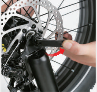
Press the quick release clamp firmly to ensure firm
