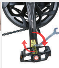
Tighten the right pedal "R" clockwise
