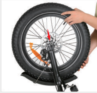
Remove the disc brake gasket
