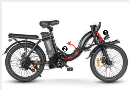
2: Fold the handle in the direction of arrow 1, open the folding buckle and fold the body in the direction of arrow 2.
